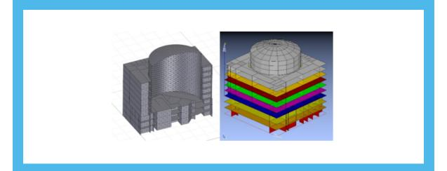
The influence of nonlinear structural behavior on the resulting floor response spectra of Systems and Components were investigated. In the next step, simplified approaches for the resulting floor response spectra will be proposed. The results will be summarised in the deliverable 6.5.
